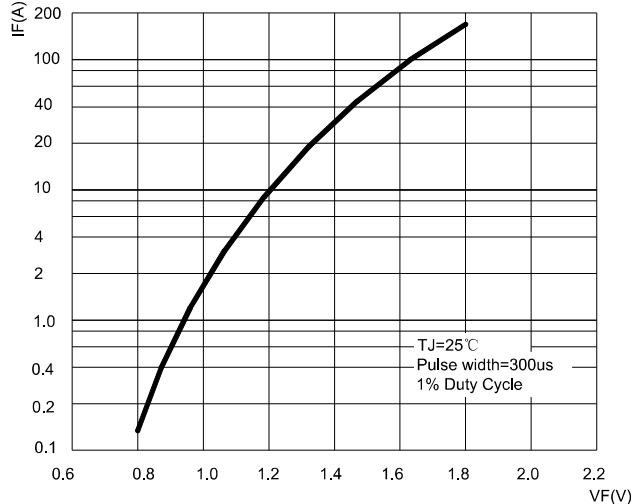
图3: 典型正向特性曲线 FIG.3: TYPICAL FORWARD CHARACTERISTICS
